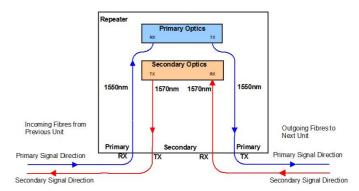
This signal will be repeated around the ring to get back to this **AMG3701R-DR-CWDMn/m** on the secondary route. As the primary input is not present on this unit, the optical signal will now be taken from the secondary optical input and retransmitted on the primary output. This action automatically maintains the integrity of the video and data transmission in the event of a fibre failure.
